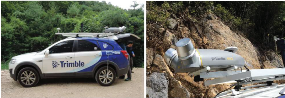
Figure 3. The vehicle equipped with Mobile Laser Scanner (MLS, Trimble MX2 model).
