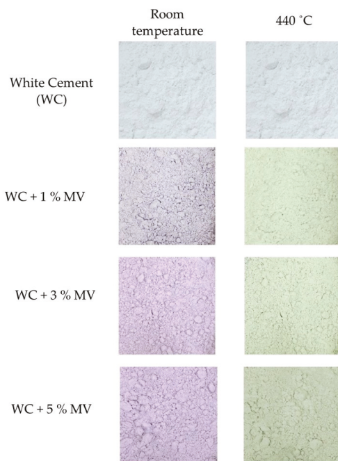
Figure 6. Color changes in the white cement and MV mixed samples exposed to different temperatures (Scale: 1000 × 1000 pixels).
