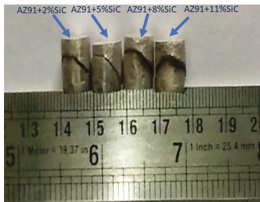
Figure 10. Fractured samples in a compression test.
