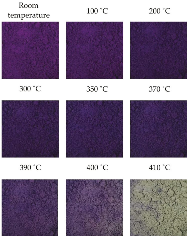
Figure 1. Color changes in the MV pigment with temperatures (Scale: 1000 × 1000 pixels).
