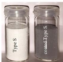
**Figure 3.** Coating of Type S spheres after a coating time of 240 min: The original spheres have a white color, the Al-coated spheres show a gray coloration.
