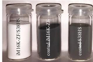
**Figure 7.** Qualitative verification of the coating of the MHGS with Setup 2: The original spheres have a white color, the coated spheres show a gray coloration.
