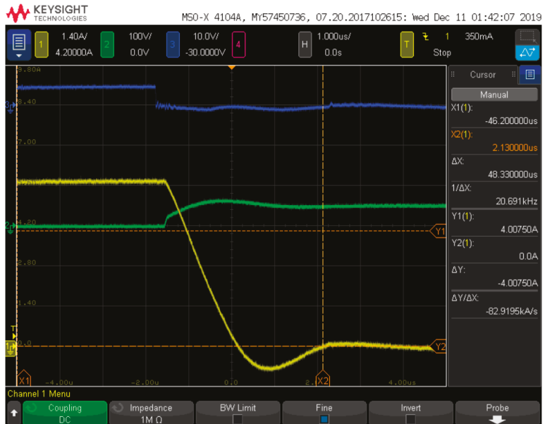
Figure 10. Total clearing time measurement setup showing time between X1 and X2.
