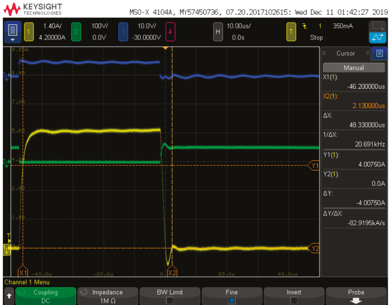
Figure 9. Trip setting measurement setup. Crossing point of cursors X1 and Y1.
