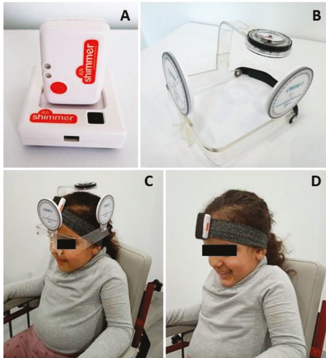
Figure 1. Devices and procedure of assessment. (A) Inertial Measurement Unit (IMU) Shimmer3 ® (Dublin, Ireland); (B) Cervical Range of Motion (CROM) 3 ® device (Lindstrom, MN, USA); (C) positioning of IMU and CROM to assess craniocervical range of motion (first assessment on the first day); (D) positioning of IMU to assess craniocervical range of motion (second assessment on the first day, and assessment on the second day).
