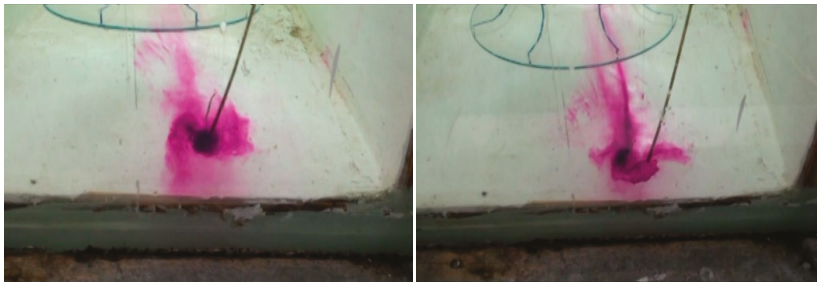
Figure 12. Backwall submerged vortex type 2 to type 3 as evidenced by the solid dye core.
