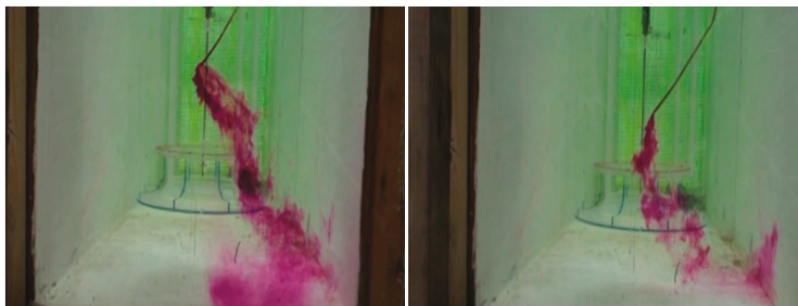
Figure 13. Flow instability and drifting behind the pump.
