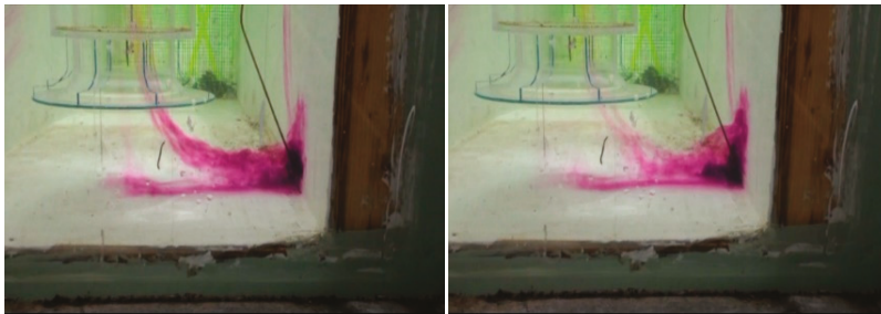
Figure 11. Intermittent side wall vortex. Type 1 to occasional type 3. Combined with the floor vortex increases the swirl along the pump column.
