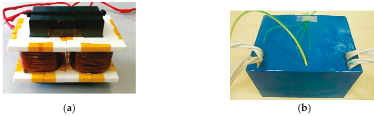
Figure 10. High Frequency Transformer (HFT) prototype. (a) Non-encapsulated laboratory developed using 3D printed bobbins. (b) Encapsulated final HFT.
