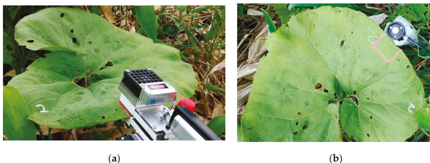
Figure 3. Measurements of (a) photosynthesis and (b) the diurnal course of incident light in the clearing site. The two panels show the same leaf. The position on the leaf lamina, at which photosynthetic traits and incident light were measured, was marked with a light-resistant ink pen (red box). In the cases when that part of the lamina was inclined, the light sensor was inclined such that the lamina and the top of the sensor were parallel to one another. Leaf mass per area (LMA) was subsequently measured by sampling the lamina part within the same red box. Photographs were taken on (a) June 21 and (b) 1 July 2020 by Kohei Koyama.
