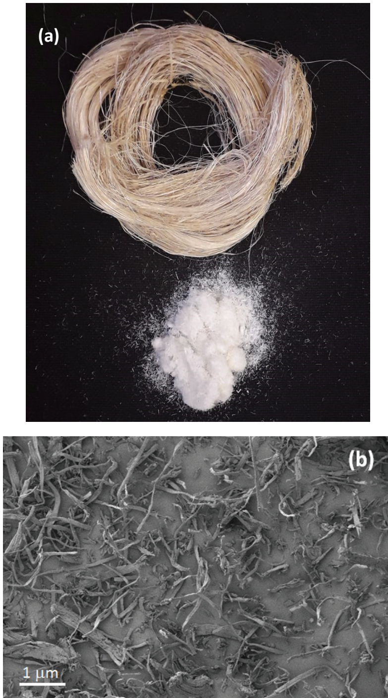
Figure 1. Fiber and cellulose nanofiber (CNF) images shows (a) photography image of raw banana fiber and extracted CNF; (b) SEM image of CNF fibrils.
