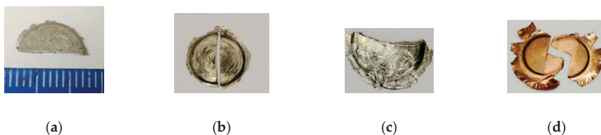
Figure 16. Optical images of samples: (a) BMG after compression only; (b) BMG after HPT for n = 1/4 revolutions; (c) BMG after HPT for n = 5 revolutions; (d) two halves of pure Cu after HPT for n = 1/4 revolutions (reprinted from [106] with permission from Elsevier).
