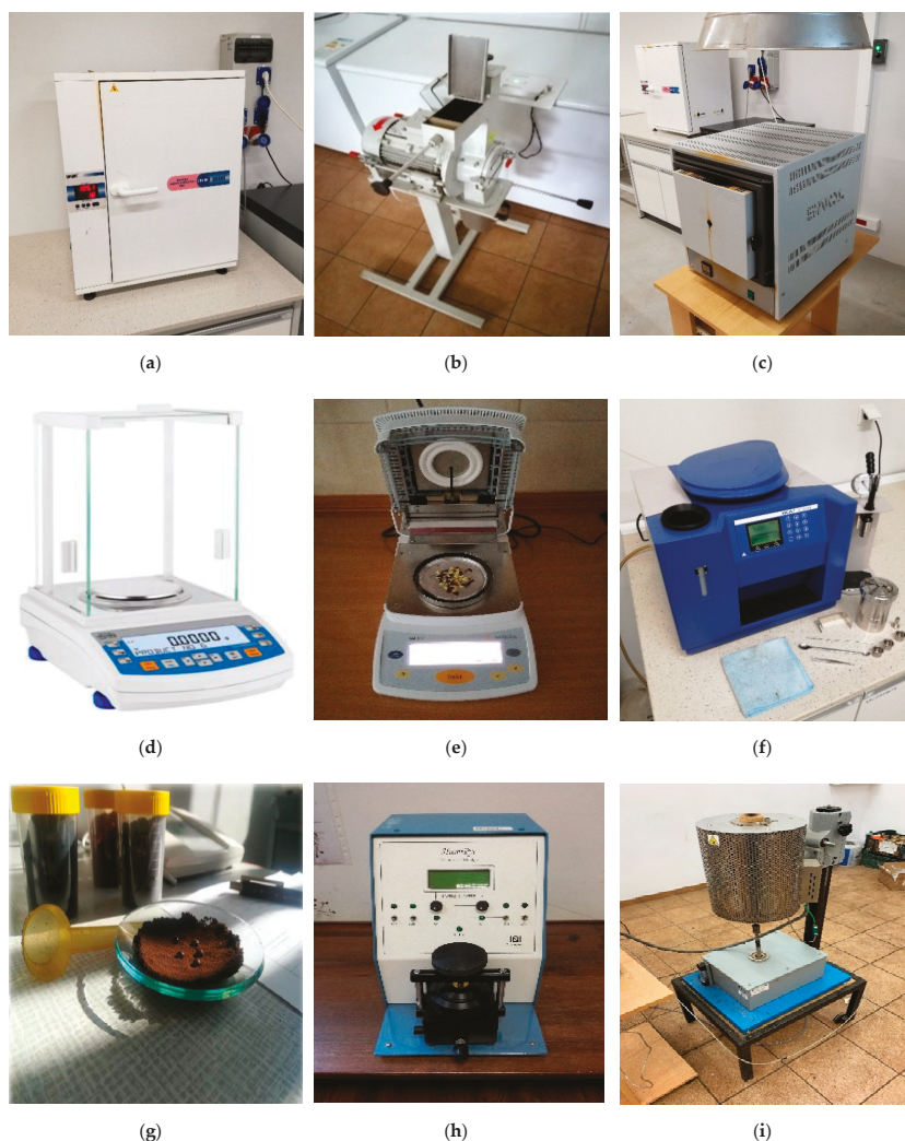
Figure 3. Laboratory devices: (a) drying chamber KBC-65W; (b) biomass mill LMN 400; (c) muffle furnace SNOL82/1100; (d) scale RADWAG AS 220.R2; (e) moisture analyzer SARTORIUS MA150; (f) calorimetric bomb IKA C200; (g) a set for WDPT (water drop penetration time) test; (h) gas pycnometer HumicPyc; and (i) thermogravimetric analyzer.
