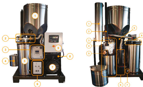
Figure 1. Pilot-scale downdraft reactor. Left: (1) Hopper, (2) Valves to flare and engine, (3) Control unit, (4) Ash vessel, (5) Gas filter, (6) Operational panel, (7) Generator, (8) Wiring box. Right: (1) Flare, (2) Exhaust stack, (3) Reactor access port, (4) Gasifier, (5) Air inlet check valve, (6) Cyclone, (7) Filter condensate drain bung, (8) Filter lid-locking lever, (9) drying bucket.
