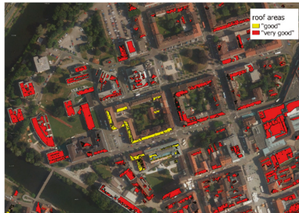
Figure 3. Example of suitable roof areas, including the classification “very good” and “good” based on data from the solar roof register [15].
