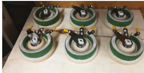
Figure 12. Resistor bank used in the electric test bench.
