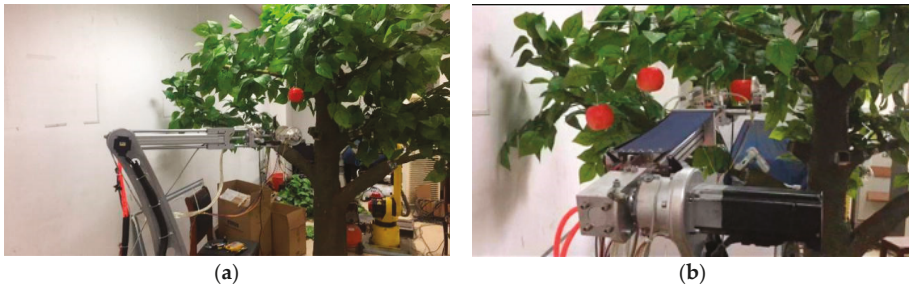
Figure 16. (a) Representing the movement process of the robot arm of apple-picking robot; (b) Representing that the picking machine recognizes the target and controls the robot arm to grasp the target through the algorithm presented in this paper.
