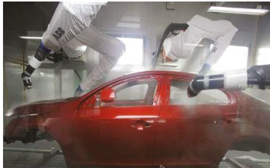
Figure 15. An automobile paint line composed by several spray-painting robots.
