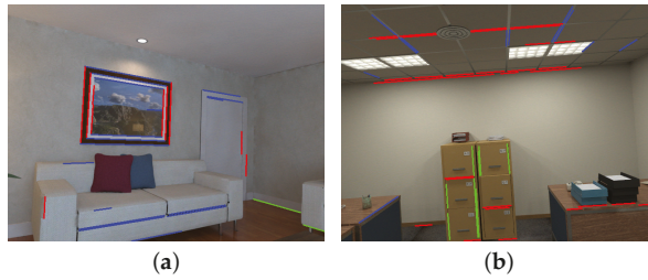
Figure 5. Results of parallel-line clustering that are used to compute vanishing directions: (a) the 120-th image in ‘Living Room 2’ sequence. (b) the 64-th image in ‘Office Room 1’ sequence. Lines with the same color are parallel in the real world. The vanishing directions obtained by these parallel lines can provide accurate and reliable constraints for MW extraction.
