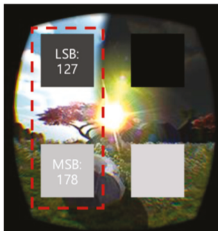
Figure 7. Example of the intensity level conversion and its inverse for measuring the current rotation angle.
