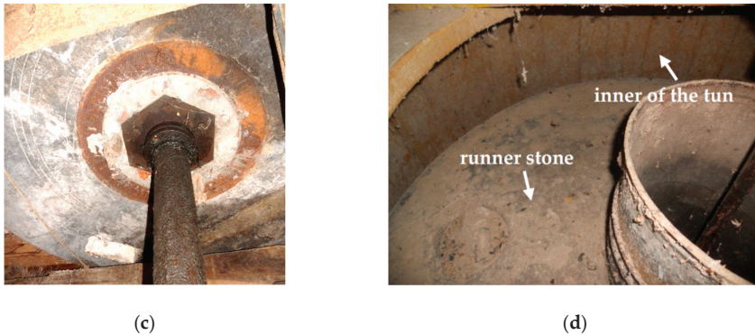
Figure 17. Coupling between the shaft C and runner stone: (a) Shaft C (Riviera mill); (b) runner stone (Riviera mill); (c) shaft C (Forno mill); (b) runner stone (Forno mill).
