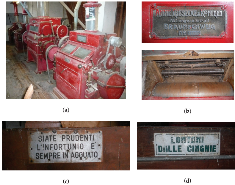
Figure 14. The Forno mill: (a) Amme Giesecke & Konegen roller mills; (b) particular of the label and inside of the mill; (c) and (d) old accident prevention signs: “Be prudent; the injury is always lurking” and “Far from the belts”.
