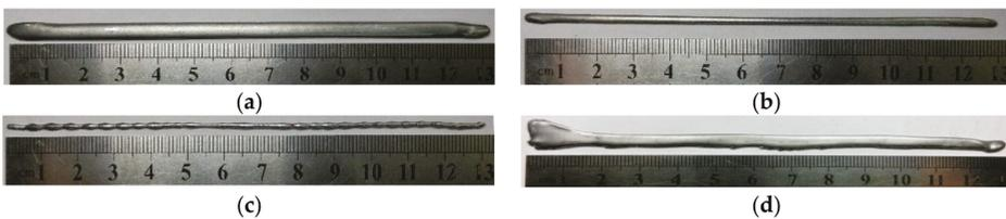
Figure 3. Various forming morphology with different combinations of process parameters. (a) Melt flowing. (b) Excellent formation. (c) Incomplete fusion. (d) Uncontrolled area.
