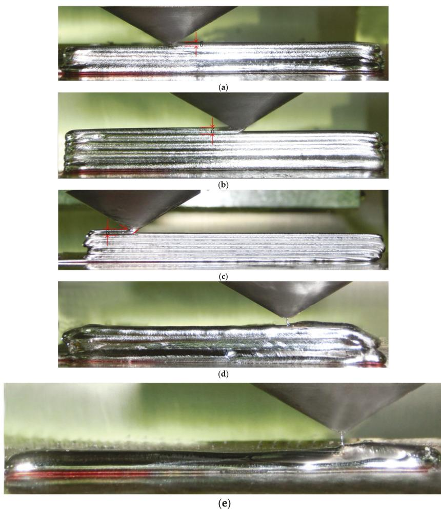
**Figure 4.** The deposited specimens in different layer thickness. (a)  $\delta = 0.9$  mm. (b)  $\delta = 1.2$  mm. (c)  $\delta = 1.5$  mm. (d)  $\delta = 1.8$  mm. (e)  $\delta = 2.1$  mm.
