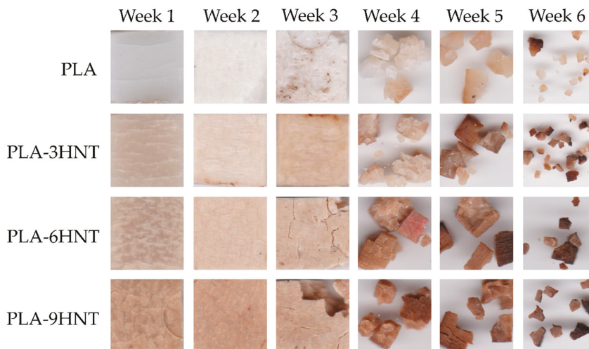
Figure 10. Optical images of the disintegration in controlled compost soil of PLA-HNT composites with different HNTs loading.
