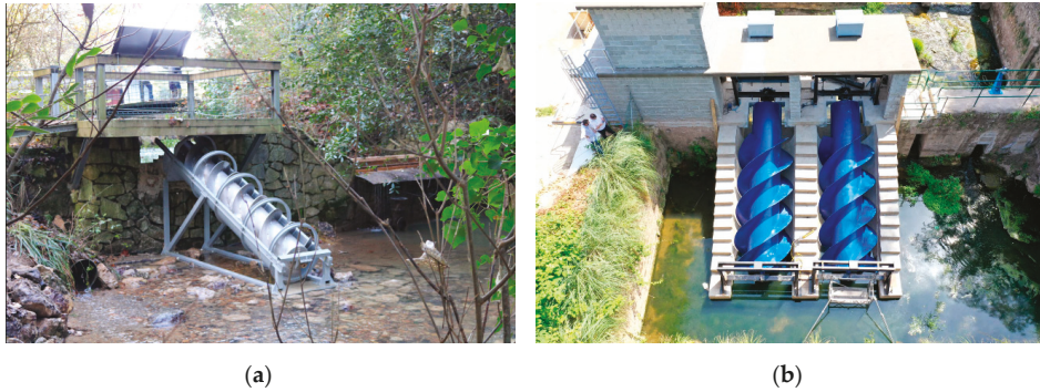
Figure 4. AST experimental prototypes. (a) Atlantic Botanic Garden of Gijón (Spain); (b) Barreda hydroelectric plant in Torrelavega (Spain).
