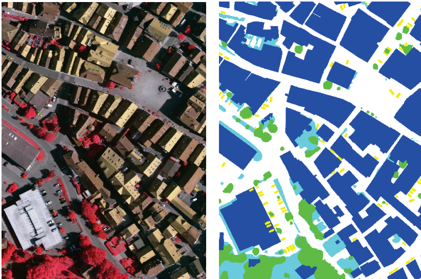
Figure 9. Sample of input scene from Figure 8 (left) and target image (right). The annotated Vaihingen corpus has five categories: tree (green), building (blue), clutter/background (red), low vegetation or LV (greenish-blue), and impervious surface or imp surf (white)
