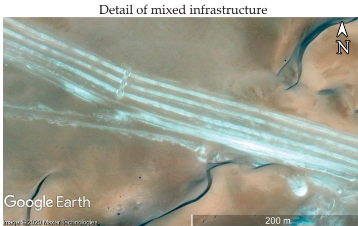
Figure 15. Close-up of a road segment in VHR optical data available on Google Earth Pro. The area corresponds with that shown by the red arrow in Figures 12–14. The road segment was not detected by the model. As evident in the figure, the road runs parallel with other infrastructure, which may have affected the ability of the model to correctly interpret the scene. The imagery date is reported to be 13 September 2013.
