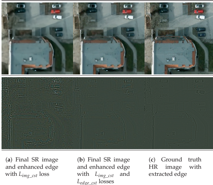
Figure 12. Effects of edge consistency loss ( L_{edge\_cst} ) on final SR (super-resolution) images and enhanced edges compared to the extracted edges from HR (high-resolution) images.
