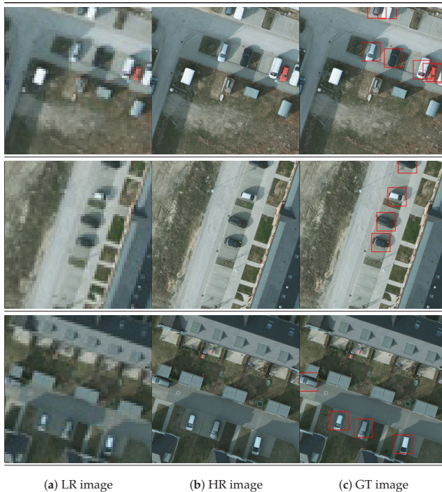
Figure 6. COWC (car overhead with context) dataset: LR-HR (low-resolution and high-resolution) image pairs are shown in (a,b) and GT (ground truth) images with bounding boxes for cars are in (c).
