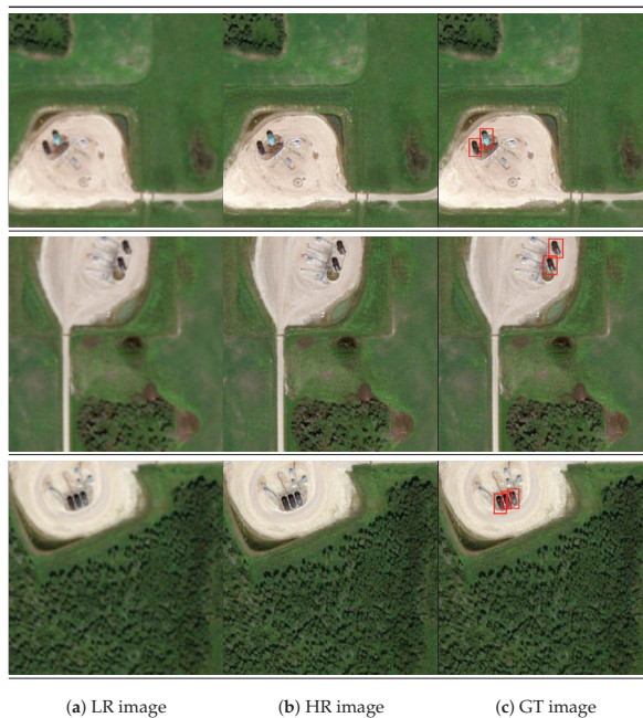
Figure 7. OGST (oil and gas storage tank) dataset: LR-HR (low-resolution and high-resolution) image pairs are shown in (a,b) and GT (ground truth) images with bounding boxes for oil and gas storage tanks are in (c).
