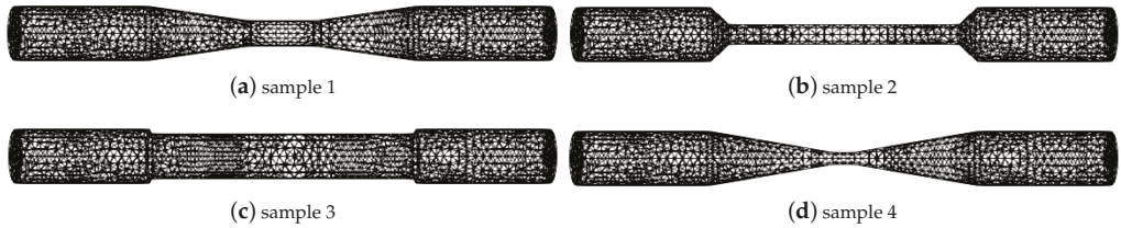
Figure 4. Four samples showing the variability in the beam geometry due to different values of the inner dimensions ( l_i, r_i ).
