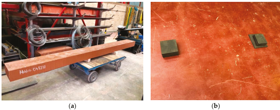
Figure 2. (a) FFU 17-06 specimens and (b) rubber cushions.
