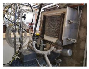
Figure 12. The Stirling motor assembly.
