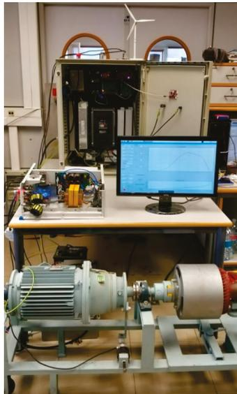
Figure 14. Experimental set up of the small wind turbine emulator system.
