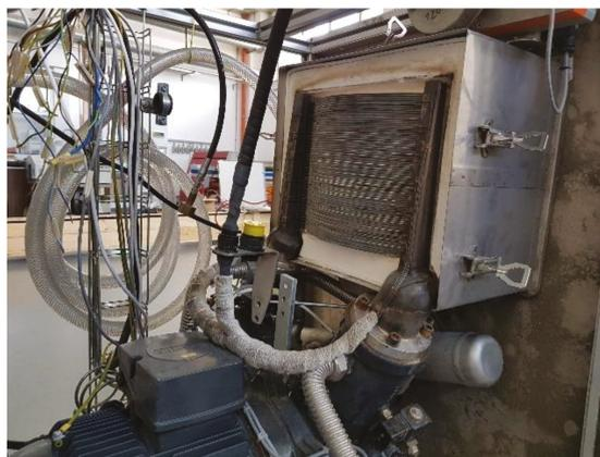
Figure 12. The Stirling motor assembly.
