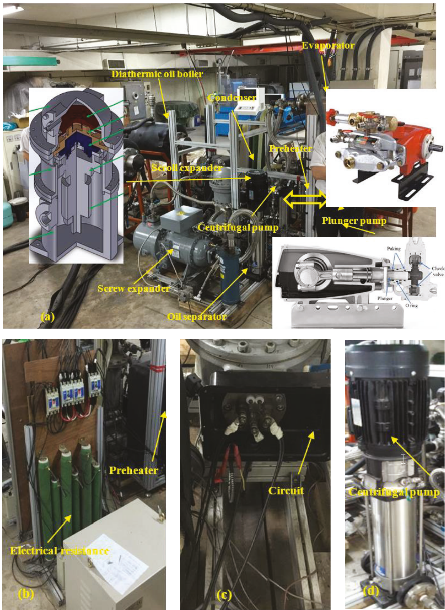
Figure 2. The pictures of (a) experimental setup; (b) the electrical load; (c) the circuit and (d) centrifugal pump.
