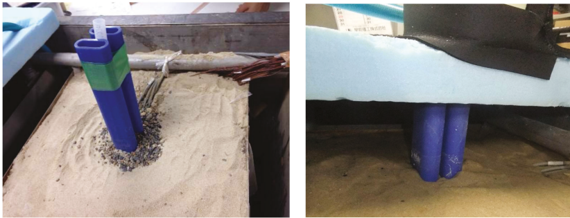
Figure 3. Photos of U-tube inside the borehole and surrounding soil.
