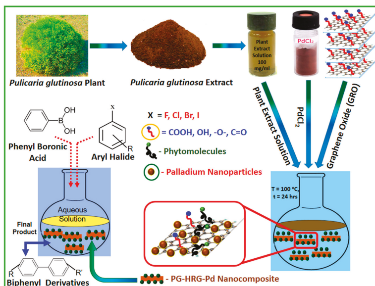
Scheme 1. Schematic illustration of the green synthesis of Pd@graphene nanocatalyst (PG-HRG-Pd) using an aqueous extract of the P. glutinosa and their catalytic activity for the Suzuki Miyaura coupling.
