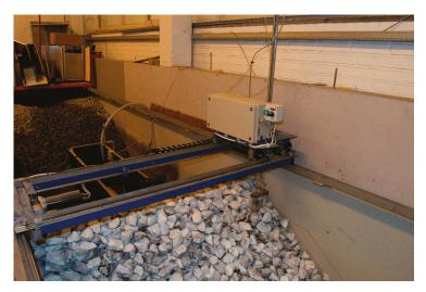
Figure 7. Profiler used to measure the eroded area.
