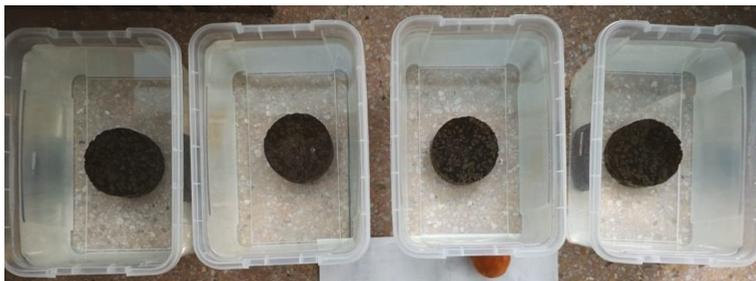
**Figure 3.** PAC-13 specimens with and without a municipal solid waste incineration-bottom ash aggregate (MSWI-BAA) used in the simulated leaching experiment.
