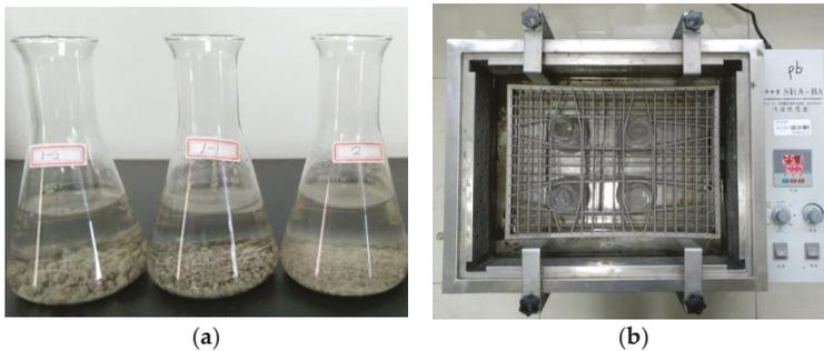
**Figure 2.** HVEP test in this study: (a) Liquid waste samples; (b) the horizontal-vibration machine.
