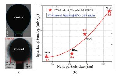
**Figure 7.** Dynamic measurement of the IFT between crude oil and nanofluids (0.1 wt.%): (a) Pendant drop method: Crude oil drop on top of a J-shape syringe needle at 20 °C (top) and at 60 °C (bottom). At 60 °C , the nanoparticles self-assembled onto the oil/water interface [16]. (b) Variation of the IFT measured with Spinning drop technique (at 60 °C) with nanoparticle size.
