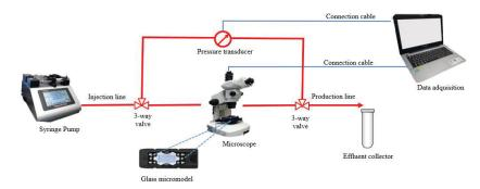
Figure 2. Diagram of the micromodel flooding setup.
