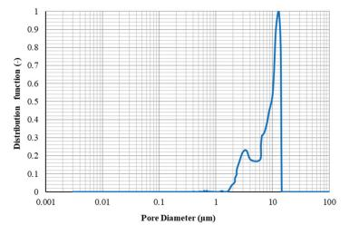
Figure 16. Pore throat size distribution for core A1.
