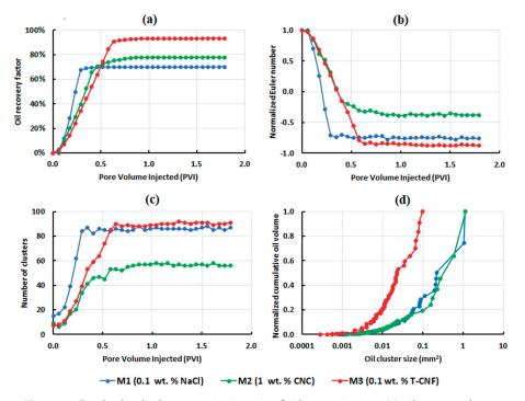
**Figure 9.** Results for the low rate injection microfluidic experiments: (**a**) oil recovery factor; (**b**) normalized Euler number; (**c**) number of clusters versus pore volume injected; and (**d**) normalized cumulative residual oil volume, as a function of oil cluster size.
