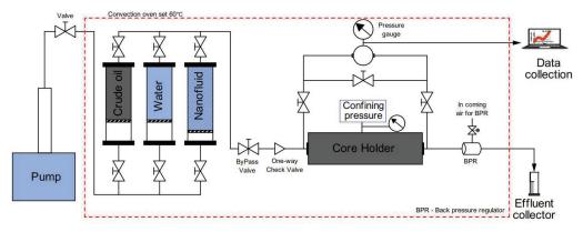
Figure 3. Schematic diagram of core flooding experiment.
