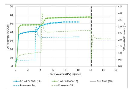
**Figure 5.** Oil recovery and pressure curves for secondary water flood (Test 1A) and secondary CNC nano flood (Test 1B). The black dotted vertical line indicates where post water flush was initiated for the nano flood. The spike in pressure curves indicates where the rate was switched from 0.3 mL/min to 3.0 mL/min, for the respective floods.
