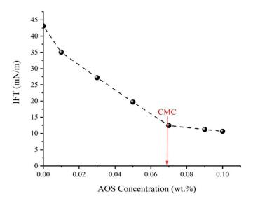
Figure 11. Crude oil-aqueous solution IFT at different concentrations of AOS surfactant.
