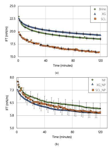
Figure 4. (a) Interfacial tension-free of NPs and (b) Interfacial tension in solutions with NPs.
