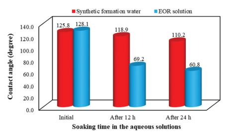
**Figure 13.** Effects of soaking time of the rock sections in red: synthetic formation water and blue: the enhanced oil recovery (EOR) solution on the oil-rock contact angle.
