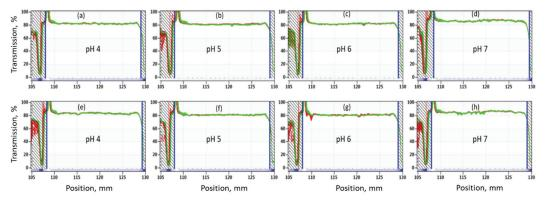
**Figure 8.** Accelerated stability analysis at 60 °C for 1 wt.% OF50-M in 3.5% NaCl brine at (**a**,**e**) pH 4, (**b**,**f**) pH 5, (**c**,**g**) pH 6, and (**d**,**h**) pH 7. The simulated stability duration was 6 months and runtime of experiment was 31 h. Samples were run in duplicate.
