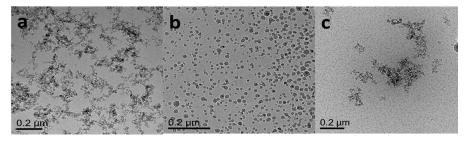
**Figure 1.** Cryo-transmission electron microscope (TEM) image of nanoparticles: (**a**) fumed hydrophilic silica nanoparticles (FNP); (**b**) amide-functionalized colloidal silica nanoparticles (ANP); (**c**) surface-modified FNP with zwitterionic polymer (FNP-MD).
