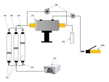
**Figure 8.** Diagram of the setup used for core flooding tests: (1) high-pressure liquid chromatographic (HPLC) pump, (2) valve, (3) distilled water, (4) synthetic formation water, (5) dead oil, (6) surfactant/nanoparticle solution, (7) core holder, (8) differential pressure transmitter, (9) calibrated burette, (10) overburden pressure.
