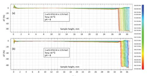
**Figure 6.** Transmission ( $\Delta$ T) profiles obtained by Turbiscan<sup>TM</sup> at 60 °C for 1 wt.% OF50-M nanoparticles in (**a**) SSW and (**b**) 3.5% NaCl brine for 1-week duration.
