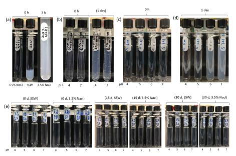
**Figure 5.** Thermal stability of 1 wt.% (**a**) OF50-UM in synthetic seawater (SSW) and 3.5% NaCl, (**b**) SBS modified particles (OF50-C1) in SSW at pH 4 and 7, (**c**) nanoparticles modified with GLYMO (OF50-C2) in SSW at pH 4–7 at 0 h, (**d**) OF50-C2 in SSW at pH 4–7 after 1 day, and (**e**) OF50-M in SSW and 3.5% NaCl brine at pH 4–7 for 30 days at 60 °C.
