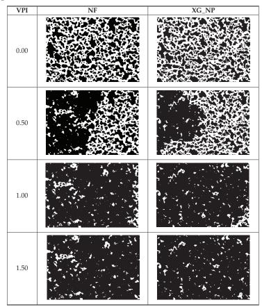
**Table A3.** Images segmented from the microfluidic tests to evaluate the effect of the flow rate on the recovery performance of the xanthan gum with NPs (XG\_NP) in comparison with the reference nanofluid (NF).
