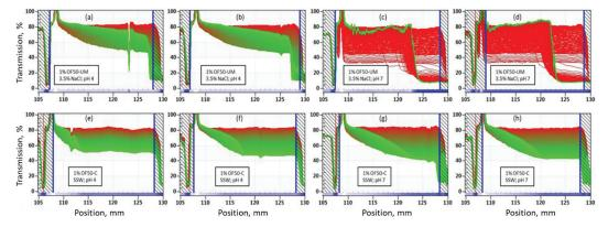
**Figure 7.** Accelerated stability analysis at 60 °C for 1 wt.% (**a**,**b**) OF50-UM in 3.5% NaCl brine at pH 4, (**c**,**d**) OF50-UM in 3.5% NaCl brine at pH 7, (**e**,**f**) OF50-C1 in SSW at pH 4, and (**g**,**h**) OF50-C1 in SSW at pH 7. The simulated stability duration was 6 months and runtime of experiment was 31 h.
