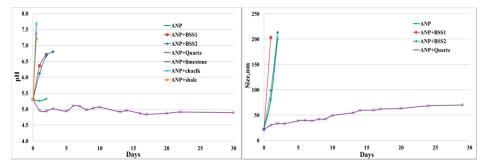
Figure 10. pH and particle size measurements for ANP suspension with different rocks.
