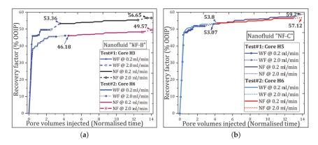
**Figure 4.** Effect of nanofluid injection on oil recovery during normal low rate and bump rate injections: (a) Sample NF-B: Test#1 the first oil production occurred  $\approx$ 1.8 PVs and the RF  $\approx$  0.5% OOIP; Test#2 produced  $\approx$  0.5% OOIP at 1 PV. (b) Sample NF-C: Test #1 the oil production occurred at  $\approx$ 2.2 PVs and the RF  $\approx$  2.3% OOIP; Test #2 the first production occurred at  $\approx$ 1.3 PV and the RF  $\approx$  0.3% OOIP.
