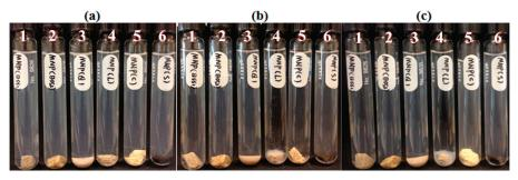
**Figure 8.** FNP-MD suspensions with reservoir rocks: (**a**), Day 0; (**b**), Day 7; (**c**), Day 30. (1: BBS1; 2: BSS2; 3: quartz; 4: limestone; 5: chalk; 6: shale).
