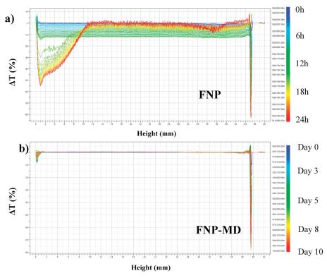
Figure 4. Delta transmission scanning results of nanofluid samples. (a): FNP (for one day); (b): FNP-MD (for 10 days).
