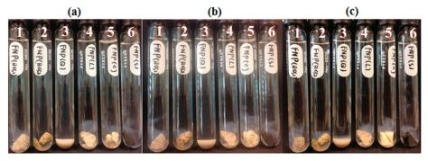
**Figure 6.** FNP suspensions with reservoir rocks: (a), Day 0; (b), Day 1; (c), Day 3. (1: BBS1; 2: BSS2; 3: quartz; 4: limestone; 5: chalk; 6: shale).
