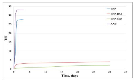
Figure 5. Turbidity scan index (TSI) results for nanoparticles suspensions.
