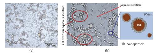
Figure 8. Visualisation of oil-in-water emulsion droplets from core flood effluent: (a)  $20 \times$  magnification image, and (b)  $50 \times$  magnification image.
