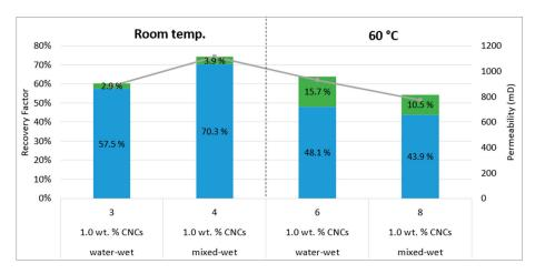
**Figure 7.** Recovery factors (% of OOIP) of tertiary recovery experiments. The vertical black dotted line acts as a marker between the experiments conducted at room temperature and 60 °C. Blue color represent the recovery factor achieved from low and high rate water flooding, while the green color denotes the recovery from the low and high rate nano flooding.
