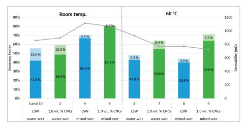
**Figure 6.** Recovery factors (% of original oil in place (OOIP)) and permeability of secondary recovery experiments. The vertical black dotted line acts as a marker between the experiments conducted at room temperature and 60 °C. Dark blue or dark green colors represent the recovery factor achieved from the low rate flooding (0.3 mL/min), while the lighter colors denote the recovery from the high rate flooding (3.0 mL/min). The numbers on the *x*-axis corresponds to the test number.
