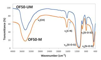
Figure 3. FTIR spectra of pristine OF50 (OF50-UM) and surface-modified/functionalized colloidal silica (OF50-M).
