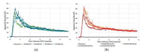
**Figure 7.** Apparent viscosity versus pore volume of the  $CO_2$  injected for the unsteady state  $CO_2$  injections into cores pre-saturated with foaming solutions containing: (a) 3500 ppm surfactant (green curves) and 5000 ppm surfactant (blue curves); (b) hybrid foaming solutions containing 3500 ppm surfactant and 150 ppm nanoparticles (orange curves) and 3500 ppm surfactant and 1500 ppm nanoparticles (red curves). The black curve is the baseline with only brine.
