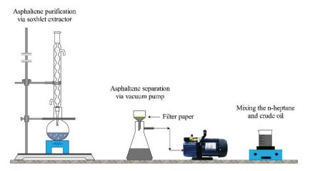
Figure 4. Schematic of the asphaltene extraction process.
