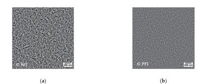
**Figure 1.** Atomic force microscopy (AFM) images of cellulose nanocrystals (**a**) and 2,2,6,6-tetramethylpiperidine-1-oxyl (TEMPO)-oxidized cellulose nanofibrils (**b**). From the images, it can be seen that both cellulose nanocrystals (CNCs) and TEMPO-oxidized cellulose nanofibrils (T-CNFs) consists of elongated particles, and that T-CNFs are longer compared to the CNCs. They both exhibit anisotropic properties. The procedure for how the AFM images were obtained is explained in Aadland [53].
