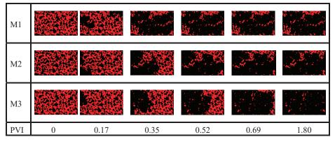
**Figure 10.** Change in the oil (in red) configuration in the analyzed part of the microchip as a function of pore volume injected (PVI) for experiment M1, M2, and M3.
