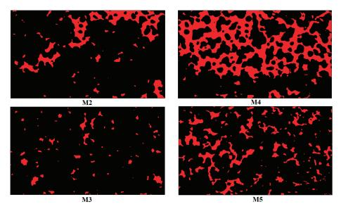
Figure 12. Illustration of the reimaging oil post flooding in CNCs experiments (M2, M4) and T-CNFs experiments (M3, M5). M4 and M5 were performed with 10 times higher injection rate, i.e., at 1.8  $\mu$ L/min vs. 0.18  $\mu$ L/min flow rate.
