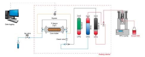
Figure 2. Schematic illustration of the experimental setup of the core flood.
