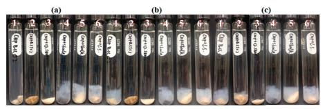
**Figure 7.** ANP suspensions with reservoir rocks: (**a**), Day 0; (**b**), Day 1; (**c**), Day 3. (1: BBS1; 2: BSS2; 3: quartz; 4: shale; 5: chalk; 6: limestone).
