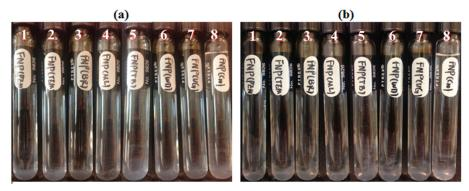
**Figure 12.** FNP suspensions stability screening with different type of oils: (a), Day 1; (b), Day 2; (1: CO1; 2: CO2; 3: CO3; 4: CO4; 5: CO5; 6: CO7; 7: CO6; 8: Decane).
