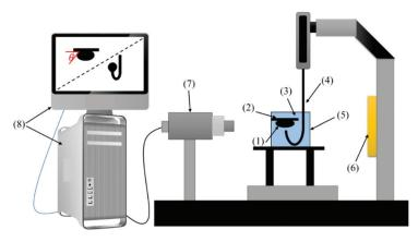
**Figure 6.** Schematic of the setup for interfacial tension IFT) and contact angle tests: (1) oil droplet, (2) rock section, (3) aqueous solution, (4) needle, (5) cell, (6) light source, (7) CCD camera, (8) processor.
