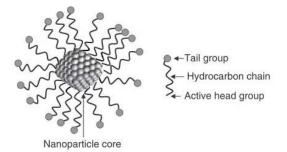
Figure 1. Schematic of a nanoparticle, showing the core and the shell [4].
