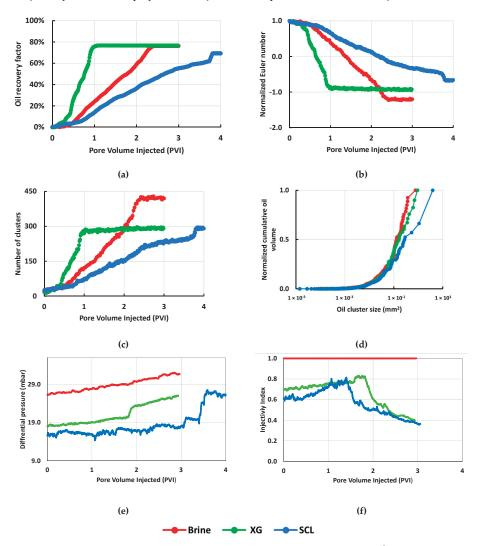
**Figure 6.** Microfluidic results for screening of biopolymer solutions at  $N_c = 1 \times 10^{-6}$ : (a) Oil recovery factor; (b) Normalized Euler number; (c) Number of clusters; (d) Normalized cumulative oil volume; (e) Differential pressure; (f) Injectivity index.
