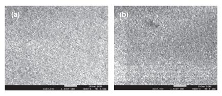
Figure 4. Scanning electron micrographs of (a) pristine OF50 and (b) OF50-M.
