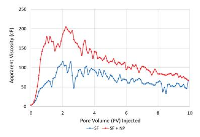
**Figure 8.** Apparent viscosity versus pore volume of the  $CO_2$  injected for the unsteady state  $CO_2$  injections in cores with residual oil ( $S_{or}$ ) and pre-saturated with a hybrid foaming solution containing surfactant and nanoparticles (SF + NP, red curve) or a foaming solution containing only surfactant (SF, blue curve).
