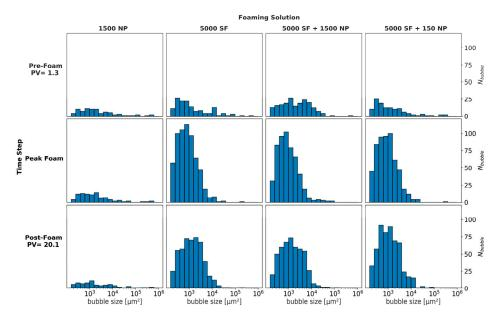
**Figure 4.** The number of bubbles (N<sub>bubble</sub>) versus bubble size for the micromodel experiments with four different foaming solutions. Foaming solutions are shown across the top and include 1500 ppm nanoparticles (1500 NP), 5000 ppm surfactant (5000 SF), hybrid 5000 ppm surfactant and 1500 ppm nanoparticles (5000 SF + 1500 NP) and hybrid 5000 ppm surfactant and 150 ppm nanoparticles (5000 SF + 150 NP).
