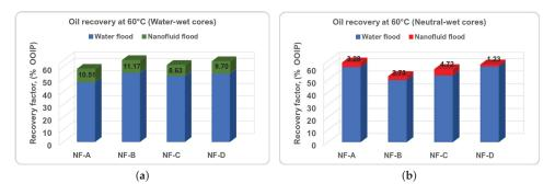
Figure 5. Comparison of average oil recoveries from various nanofluid floods: (a) Water-wet cores [16], and (b) Neutral-wet Berea core (present study).
