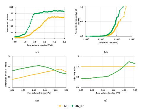
**Figure 8.** Microfluidic results showing the effect of a higher flow rate (0.39 μL/min) on the recovery performance: (**a**) Oil recovery factor; (**b**) Normalized Euler number; (**c**) Number of clusters; (**d**) Normalized cumulative oil volume; (**e**) Differential pressure; (**f**) Injectivity index.
