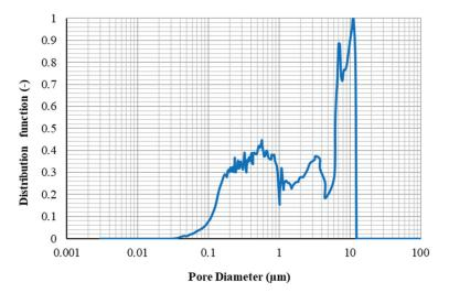
Figure 17. Pore throat size distribution for core A2.
