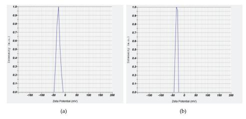
Figure 9. Zeta potential measurements for (a)  $SiO_2$  and (b) alpha olefin sulfonate (AOS) +  $SiO_2$  solutions.
