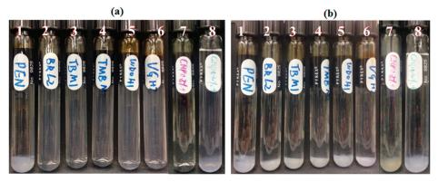
**Figure 14.** ANP suspensions stability screening with different type of oils: (**a**), Day 1; (**b**), Day 3; (1: CO1; 2: CO3; 3: CO5; 4: CO2; 5: CO7; 6: CO6; 7: CO4; 8: Decane).
