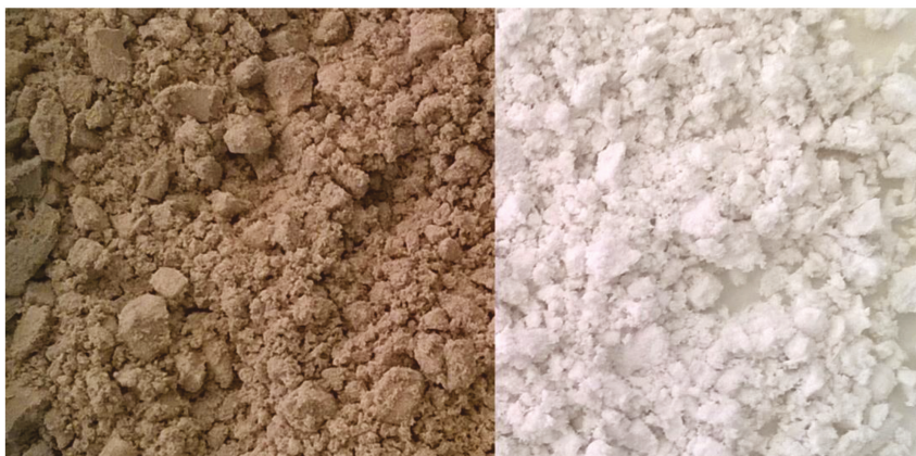
Figure 4. Side-by-side comparison of dry solids obtained without activated carbon treatment ( left ) and with activated carbon treatment ( right ).
