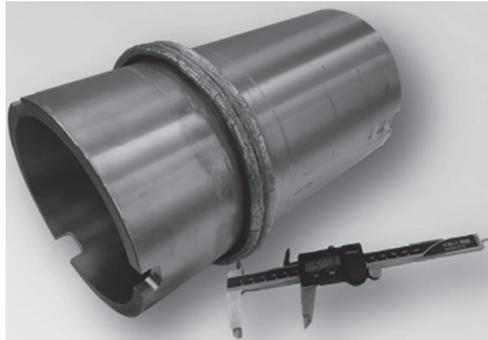
**Figure 18.** Medium-size friction welded Mo-tube (OD: 150 mm, ID: 130mm) [46].
