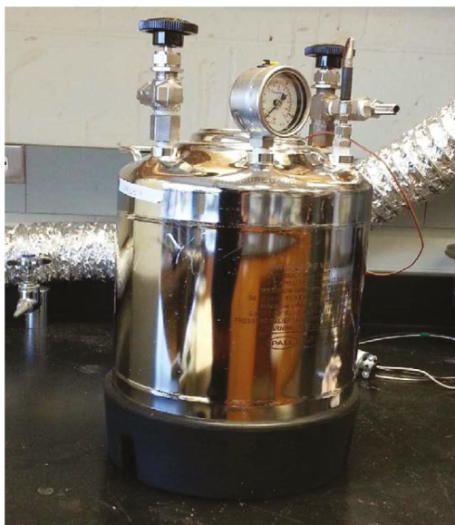
Figure 1. Ammoniation reactor with internal volume of 3 L.
