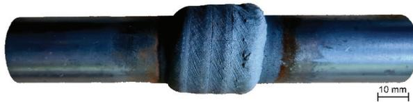
Figure 7. Welding seam after cladding by PTA.
