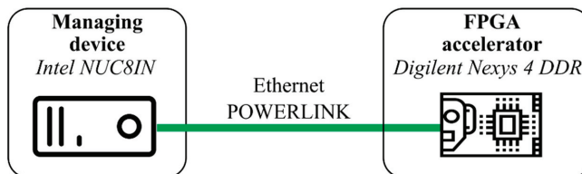
Figure 12. Hardware architecture used for forecasting algorithms implementation.
