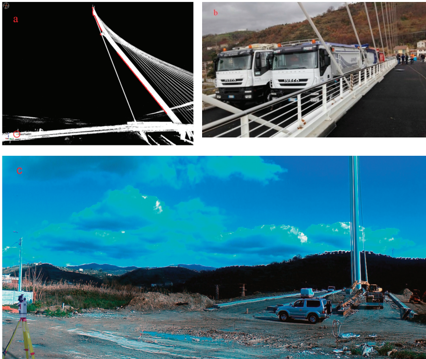
Figure 17. The Test on the San Francisco Bridge: (a) The Layout with the TLS position (red circle) and the scanned line (red line); (b) Trucks used as loads; (c) The TLS, positioned after the alignment operation, preliminary to the test.
