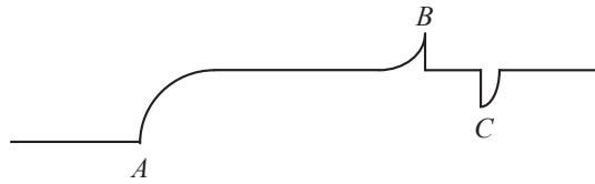
Figure 2. Illustration of the edge point and noise point.
