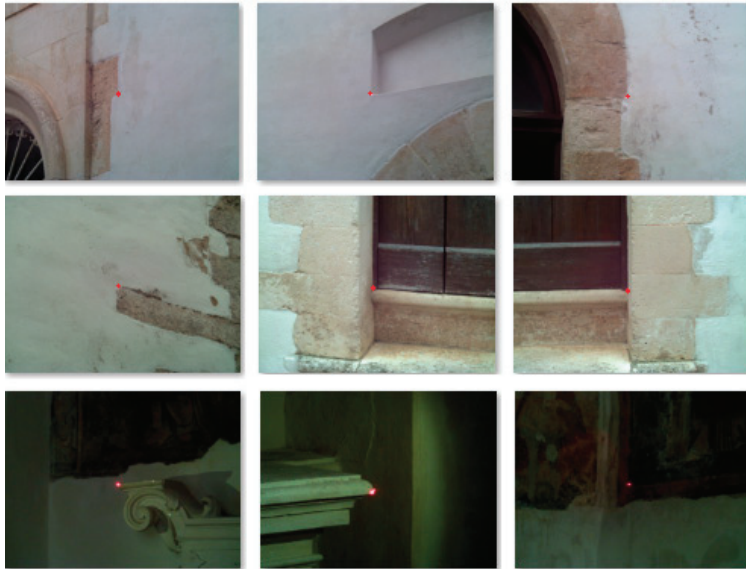
Figure 4. Images of some ground control points used for the georeferencing of the point cloud.
