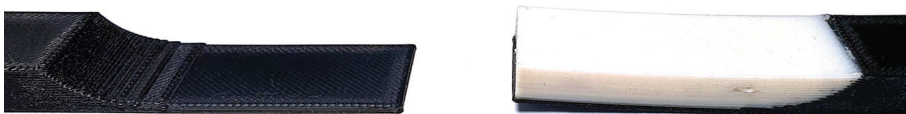
Figure 1. Tip of Acoustic Black Holes (ABH) beam with (right) and without (left) additional damping material.
