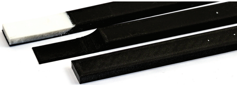
Figure 2. Overview of beam specimens with different system complexity: simple beam structure made of PLA ( front ), beam structure with an ABH made of PLA ( center ), and beam structure with an ABH made of PLA with an additional damping treatment made of an thermoplastic polyurethane ( back ).
