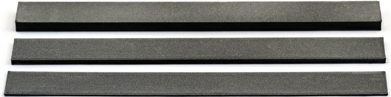
Figure 3. Overview of investigated specimen of three different thicknesses (6 mm, 3 mm, 1 mm).
