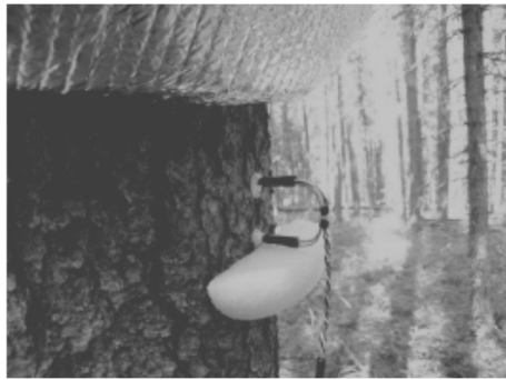
Figure 2. Thermal Dissipation Probes (TDPs) installed in a boreal, coniferous tree with the isolation material (upper part of the picture) ready to cover the sensors and protect them from direct exposure to solar radiation that could affect the sensors' temperature.
