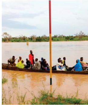
Figure 7. Colored hydrometric staff at Garbey Kourou, Niger.
