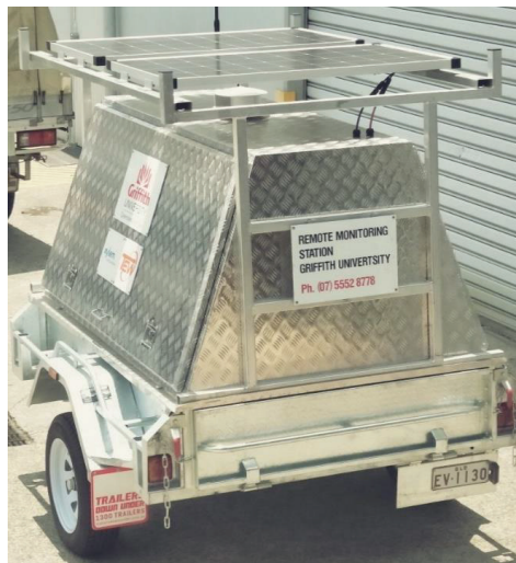
Figure 1. Trailer exterior modified with solar panels.
