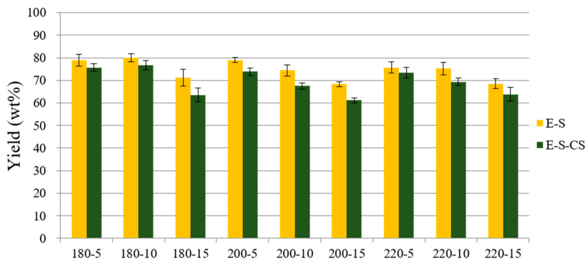
Figure 2. Yields of the solid fractions from steam explosion and organosolv treatment of EFB under different temperatures and residence times.
