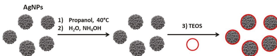
Figure 12. Modified Stöber method for coating of AgNPs with silica.
