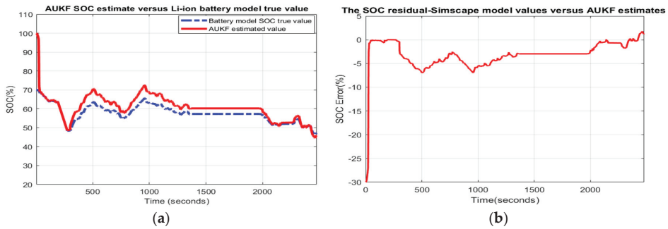
Figure 8. Robustness to simultaneous changes, SOCini = 1, Qnom = 4.2 Ah (ageing effects); (a) AUKF SOC value versus battery model true value; (b) SOC residual.
