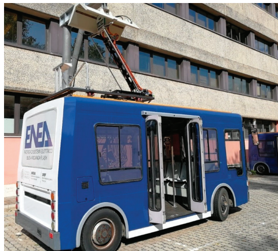
Figure 9. Charging phase of the prototype of P3 with flash charging technology.
