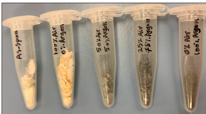
Figure 1. Color changes in electrospun titanium oxide (TiO 2 ) nanofibers (NFs) in argon-air mixtures.
