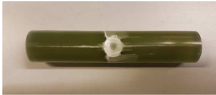
Figure 8. Long axial crack on top of sample A1, with an indentation caused by a crosshead of the strength testing machine.
