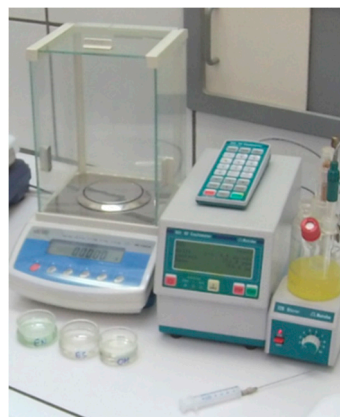
Figure 5. Instrument for measuring water content by Karl Fischer coulometric titration method.
