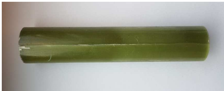
Figure 9. Long axial crack in the lower part of sample C1.
