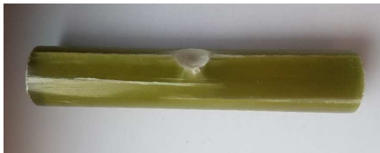
Figure 10. Indentation at the point of operation of the crosshead of the strength testing machine, long axial crack and cracks on the side surface of sample C3.
