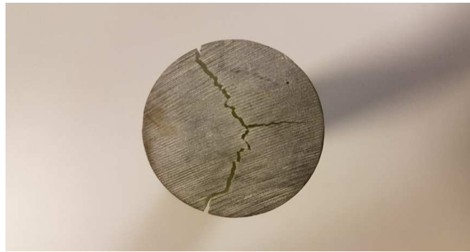
Figure 11. Cracks on flat side surface of sample C4.
