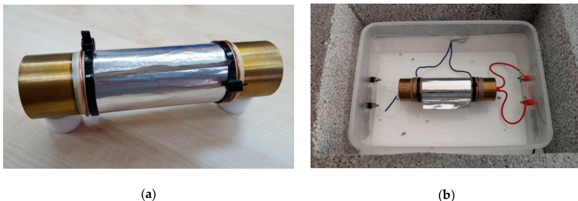
Figure 4. Photograph of the insulation sample prepared for testing: (a) zoom on sample; (b) after placing the sample in the measuring system.
