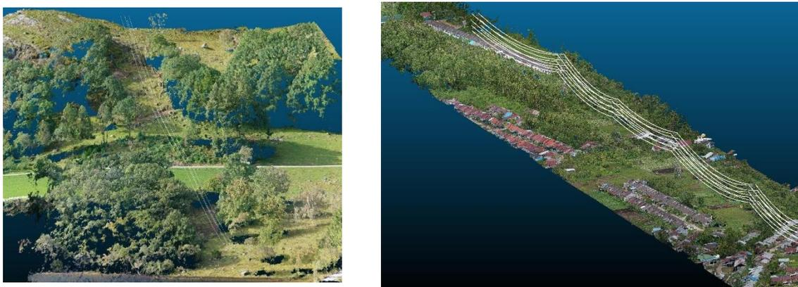
**Figure 1.** A visualization of the goal of the research, i.e., the results of the 3D reconstruction of power lines (source: FlyTech unmanned aerial vehicle (UAV) test flights)—power line over the UAV-derived point cloud representation of the digital surface model (DSM).
