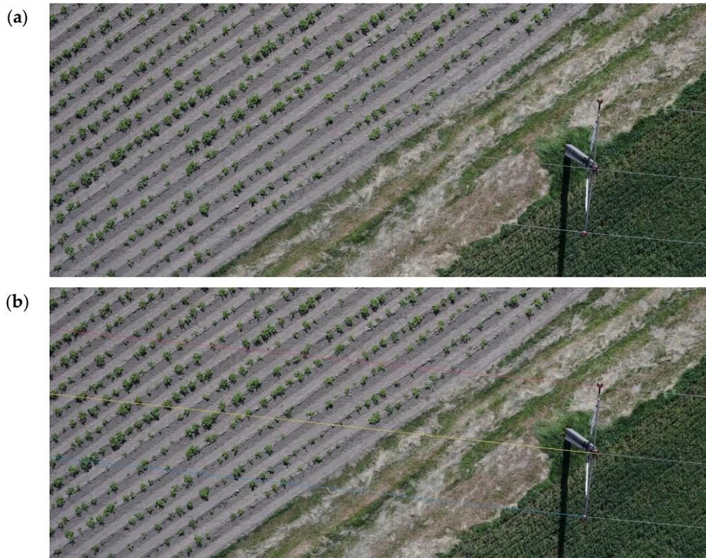
**Figure 16.** Detection results of the wires: (a) original image; (b) processed image with highlighted wires detected.
