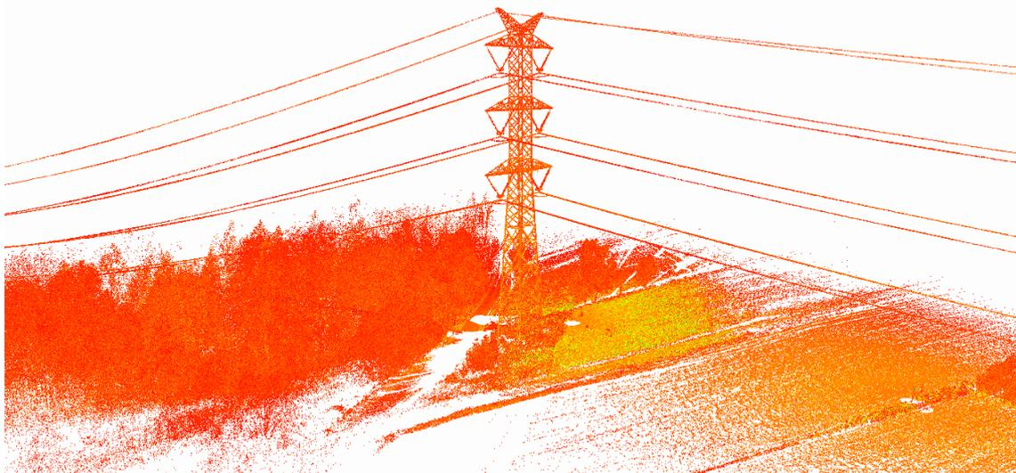
**Figure 15.** High-resolution terrestrial laser scanning (TLS) point cloud of a high-voltage power line (Dataset IV). The color of the points is determined by the intensity (the strength of the reflected laser beam).
