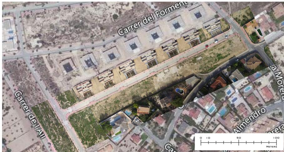
Figure 10. Image of the final orthophoto superimposed on the Google Maps satellite image.
