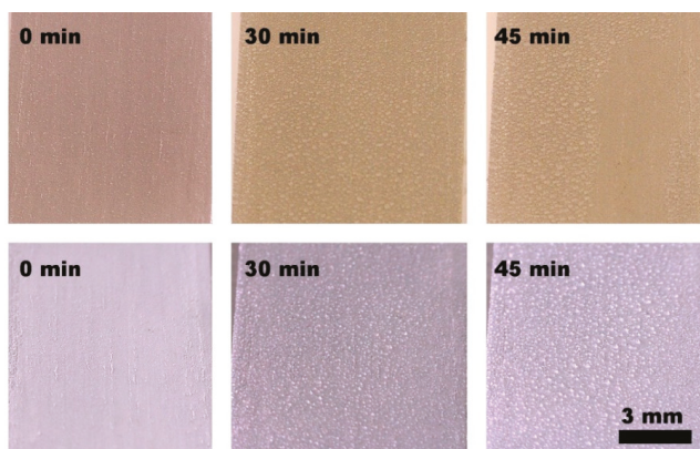
Figure 15. Condensation of water droplets on to superhydrophobic coating. The top images correspond to a tilt of 90^\circ while the bottom images are from the sample tilt 45^\circ . All the images have the same magnification.
