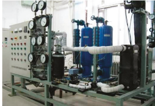
Figure 5. The test-bed of a compression refrigeration system.
