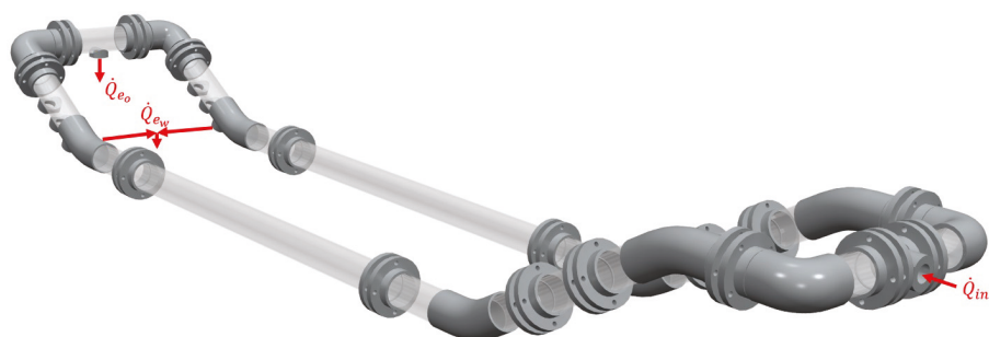
Figure 1. The Multiple Parallel Pipe Separator (MPPS) prototype.
