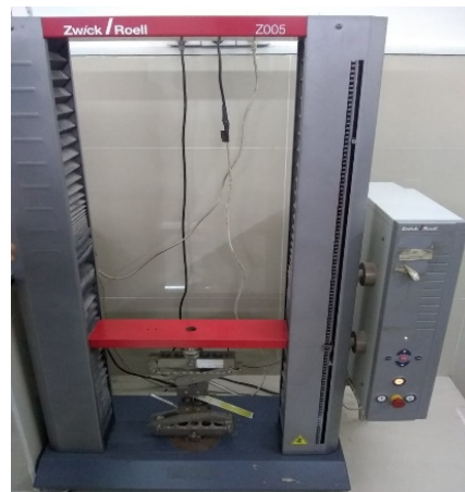
Figure 2. A 5 kN universal tensile testing machine.
