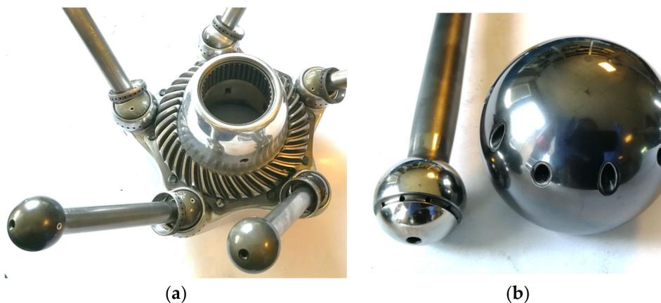
**Figure 4.** High capacity spherical plain bearings used in PAMAR engine designs: (a) wobble plate—connecting rod assembly of PAMAR 3 engine; (b) size comparison between the bearings used in PAMAR 4 and PAMAR 5 engines.
