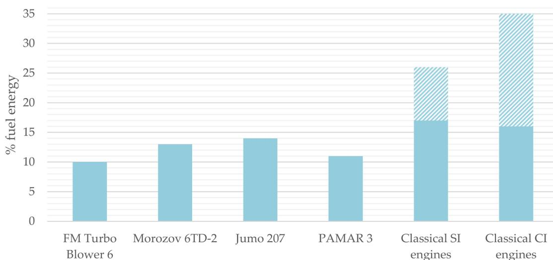
**Figure 8.** Heat loss to the cooling system of historical opposed piston engines [18] compared with the classical SI and CI designs [15]. The comparison applies to the CI OP2S engines: FM Turbo Blower 6 (1938)–102 dm<sup>3</sup>; Morozov 6TD-2 (1967)–16,3 dm<sup>3</sup>; Jumo 207 (1939)–16,6 dm<sup>3</sup>; PAMAR 3 (2006)–3 dm<sup>3</sup>.
