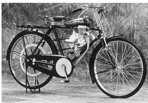
**Figure 13.** Soichiro Honda motorcycle (1947 Honda A-type—adapted from [world.honda.com](http://world.honda.com)).
