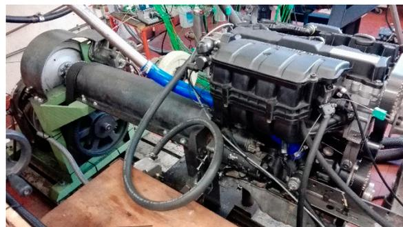
**Figure 2.** TU5 JP4 engine and Telma CC-125 dynamometer.
