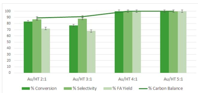
**Figure 6.** Comparison of the performance in furfural oxidation of Au/HT catalysts with supports having different molar Mg: Al ratios. Batch reactor,  $p = 6$  bar ( $O_2$ ),  $t = 110$  °C, 2 h, 600 rpm, FF/Au molar ratio = 200:1, [FF] = 26 mM, 25 mg of catalyst.
