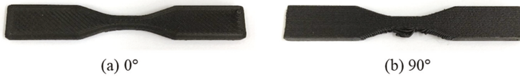
Figure 9. Examples of the impact of build orientation on dimensional accuracy. (a) 0°; (b) 90°.
