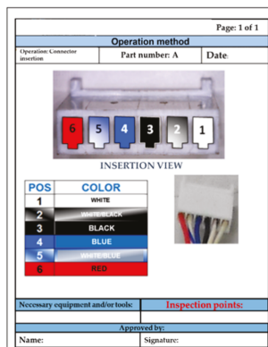
Figure 6. Provisional aid for cable insertion.
