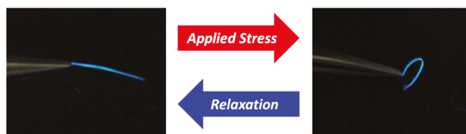
Figure 5. Photograph of elastic bending of the light-emitting elastic organic crystal of 1 . Reproduced from [15] with permission of Wiley-VCH Verlag GmbH & Co. KGaA, Weinheim, copyright 2016.
