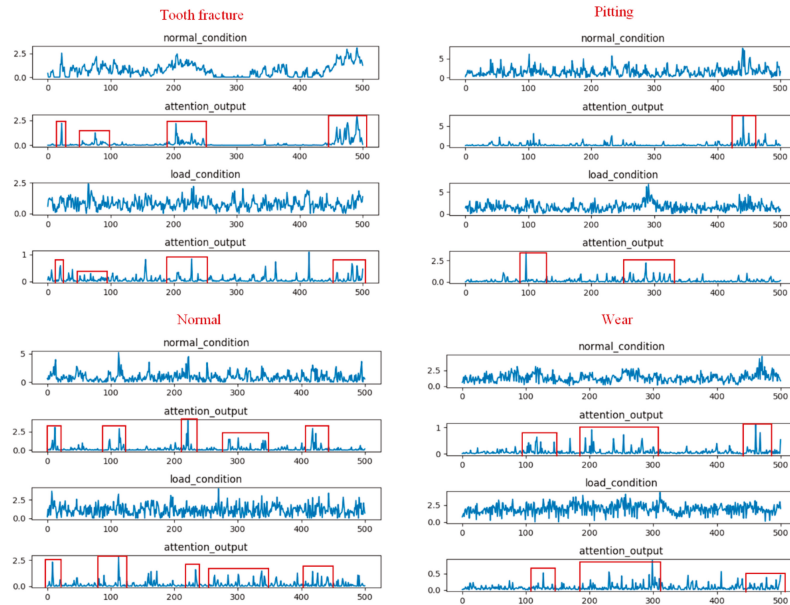
Figure 10. Visualization results of randomly selected filters from the multi-scale pool layer and temporal attention output for four different types of raw gear signals under the two load conditions corresponding to the attention based multi-scale CNN model for evaluation B.
