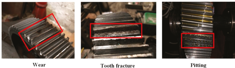
Figure 6. Fault pattern of the gears.
