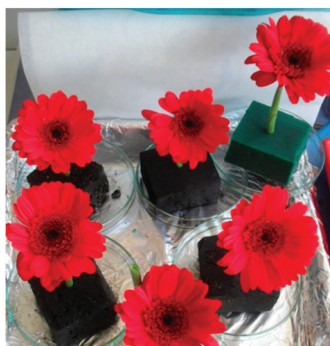
Figure 10. Appearance of cut flowers (Transvaal daisies, Gerbera spp) on a tannin–furanic foam (black) compared to a synthetic phenol–formaldehyde/furanic foam (green).
