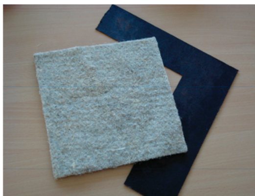
Figure 17. A nonwoven web of hemp fibers and the composite obtained by impregnation with a tannin–furanic resin.
